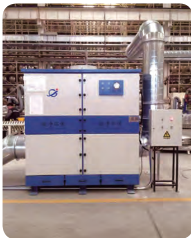
High power purification equipment for dust removal is used in Minghui Tianhai
